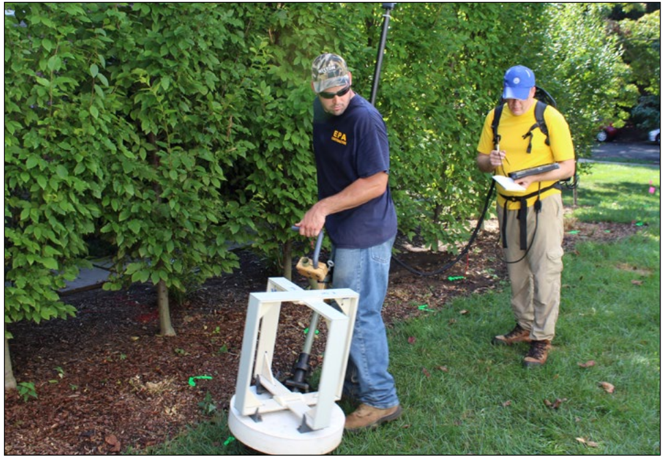
Manned Portable Vector, or MPV, technology seen here was proved to be effective and is being used during ongoing munitions investigation work in Spring Valley.
