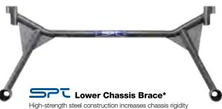
by connecting the subframe to the engine cross member.
