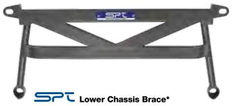
High-strength aluminum construction increases chassis rigidity by connecting the subframe to the engine cross member.
