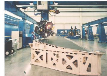
Can produce parts with modest curvatures
