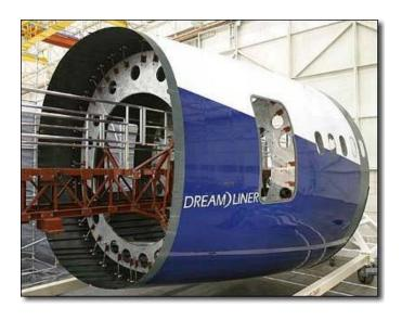
Boeing 787 fuselage barrel sections produced using an automated fiber placement machine designed/built by Electroimpact (Mukilteo, WA)
