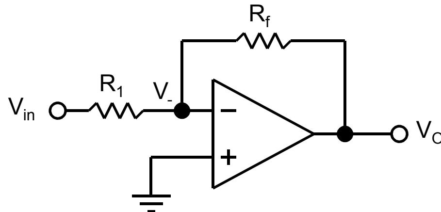
$$\left. \begin{aligned} V_o &= A(V_+ - V_-) \rightarrow V_- = -V_o / A \\ (V_{in} - V_-) / R_1 &= (V_- - V_o) / R_f \end{aligned} \right\} V_o = \frac{-R_f / R_1}{1 + (1 + R_f / R_1) / A} V_{in}$$
