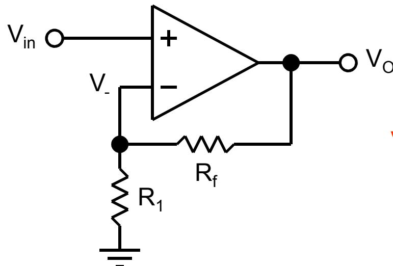
$$V_o = \frac{A}{1 + \frac{R_1}{R_1 + R_f} A} V_{in}$$
