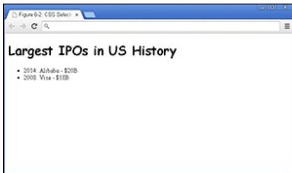
Figure 6-2: CSS targeting the heading h1 element.
