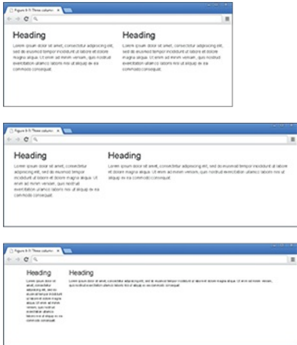
Figure 8-7: A two-column site displayed on tablet, desktop, and large desktop.
