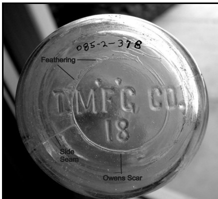
Figure 2-36 – Base showing Owens machine scar (California State Parks collection)
