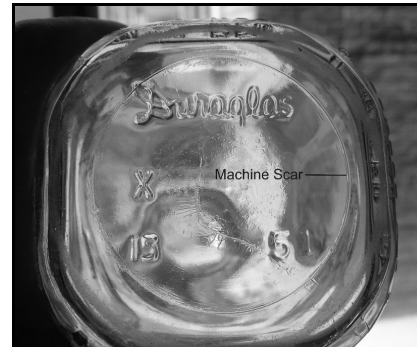
Figure 2-37 – Base showing later machine scar
