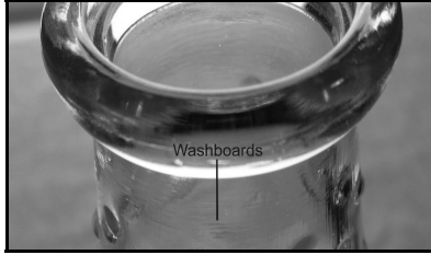
Figure 2-32 – Washboards on neck created by the press-and-blow machine process
