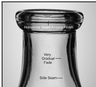
Figure 2-31 – Finish created by the press-and-blow machine process
