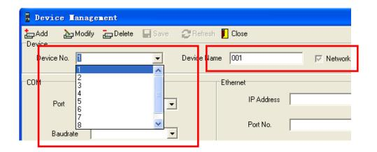
**4.4** For TCP/IP connection, select "Network". And then specify the "IP Address", The "IP Address" should be same as the one in Fingerprint. The model No. pls confirm with your Supplier. (Notes: for details of the IP configuration, please refer to the Fingerprint **Hardware Manual section 7.6**)
