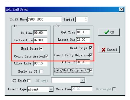
**11.1.7 Allow Late**: A buffering time zone for late arrival. In this example, the setting is 00:15, which means 15 minutes buffering time is provided. For staff arriving at 09:15 or before, the system will not count the staff as late arrival. However, if staff arrival at 09:16, then the staff is late, and the late time will be 16 minutes, instead of 1 minute.
