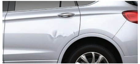
Hail damage or punctures on any panel
