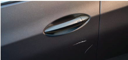
1 dent or 2 scratches (equal to or less than 4”) per panel
