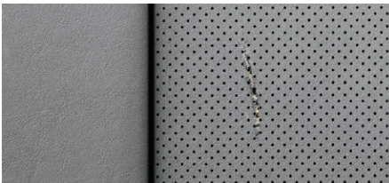
Tears equal to or less than 1/2"
