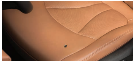
Upholstery holes more than 1/8"
