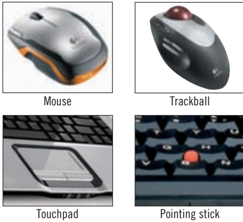
FIGURE A-6: Pointing devices
