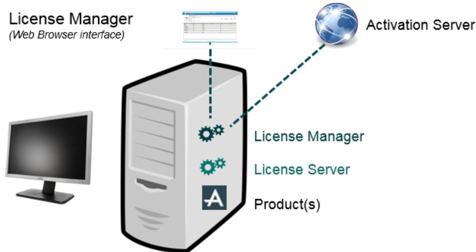
In this sample topology, a single node system, the product machine has both the License Server and License Manager components.
