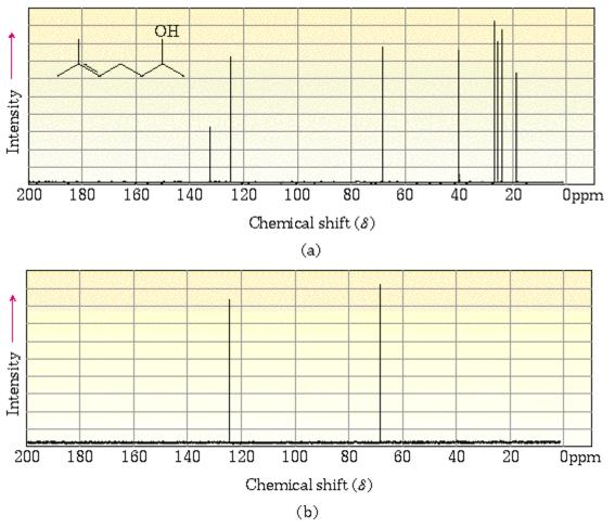
In a) all carbons are seen, in b) only CH carbons show, in c) positive signals are seen for CH and CH<sub>3</sub> and negative peaks are seen for CH<sub>2</sub>
