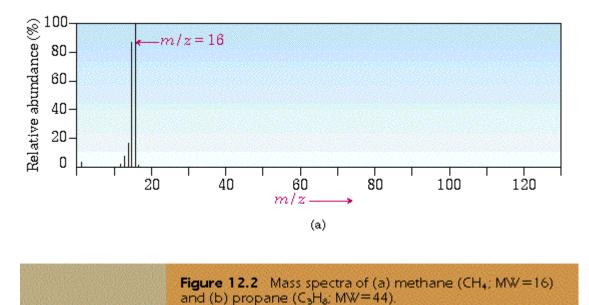
Parent or molecular ion (M+) = The ion of the compound with only the loss of the electron. Usually the heaviest peak in the spectrum.
