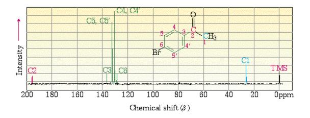
Notice that in these spectra that the peak heights for single carbons are not the same. And no attempt has been made to integrate them. This is because integration does not work for time averaged spectra.
