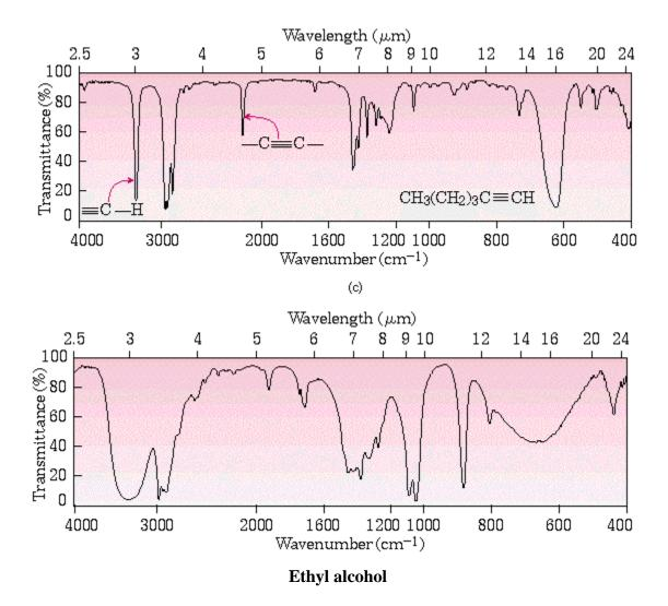
The fingerprint region is that area below 1600 wavenumbers which is ordinarily too complex to be diagnostically useful. The fingerprint region can be interpreted but is principally used to compare individual compounds to one an another for identification of the compound, hence the name fingerprint.
