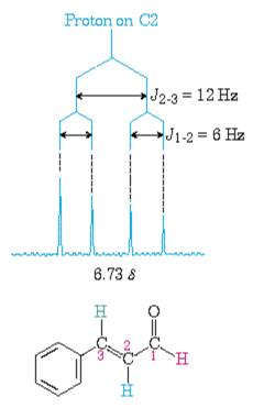
The amount by which the signal is split (the distance apart) is called J, the coupling constant but is not critical for our level of understanding. Hydrogens splitting each other have the same J value.
