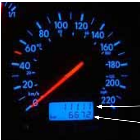
A: Main Odometer B: Short trip Odometer
