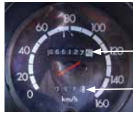
C: Main Odometer D: Short trip Odometer
