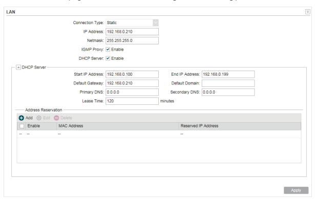
1. For LAN connection type, the device only supports Static.
