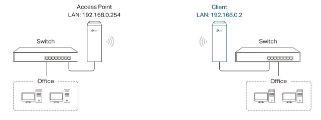
Network requirements: Help the wired devices to connect to the wireless network.
