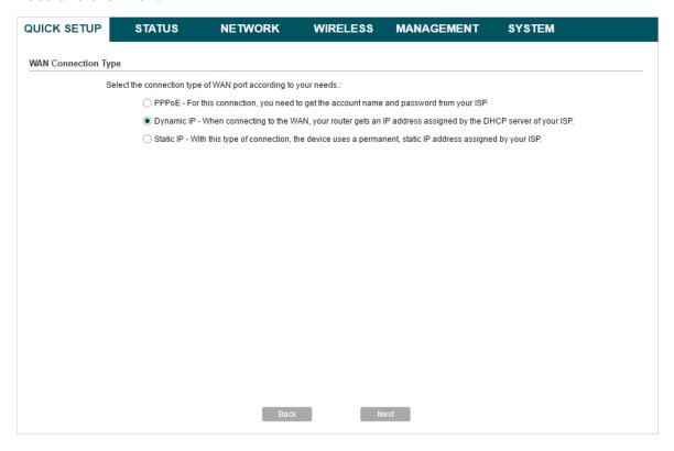
The device supports types, *PPPoE*, *Dynamic IP* and *Static IP* for the WAN connection. You can contact with your ISP to confirm your WAN connection type.
