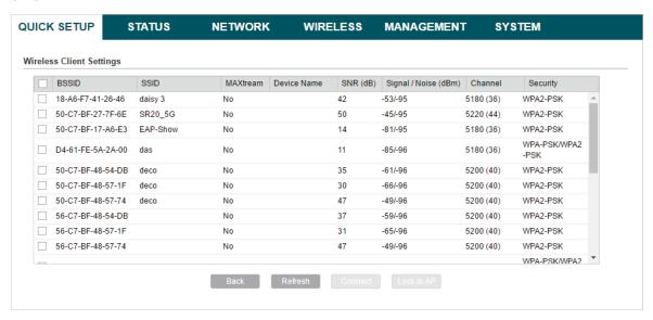
5. In the **Wireless Client Settings** section, specify the wireless parameters to connect to the specified wireless network. Click *Next*.
