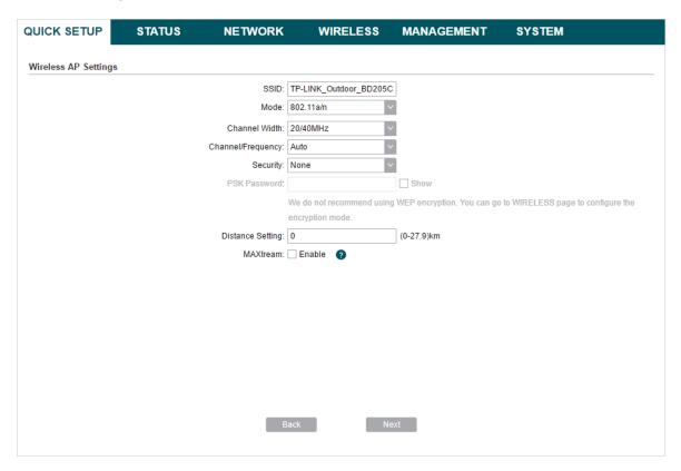
4. In the **Finish** section, review the configurations and click *Finish* to complete the quick setup.
