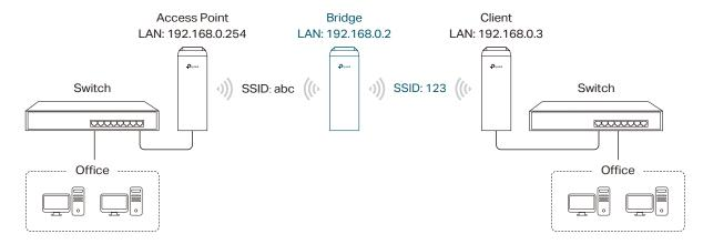
**Network requirements:** Extend the wireless network to eliminate the wireless signal-blind areas. Users can use different SSID and encryption type from those of the root AP device to access the network.
