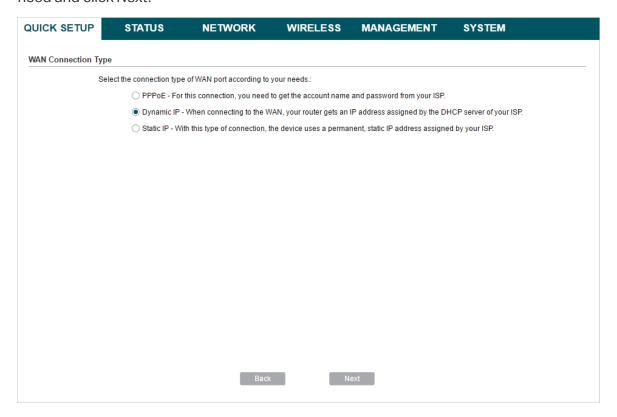
The device supports three types of the WAN connection, including *PPPoE*, *Dynamic IP* and *Static IP*. You can contact with your ISP to confirm your WAN connection type.
