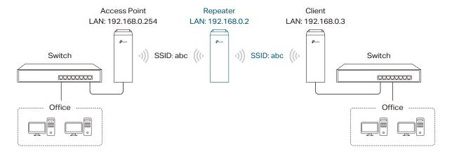
Network requirements: Repeat wireless signal and extend the wireless network coverage.
