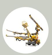
Used for drilling new high speed railway links across the world and equipped with our remarkable hydraulic rock drills, face drilling rig **Boomer** range represents a major leap forward in productivity and economy. And thanks to the state-of-the-art computer controlled drilling system, all four of the rig's booms can be supervised by a single operator. This marks a new milestone in low cost drilling.
