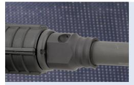
A red polymer Accu-wedge (below l.) reduces play between the upper and lower receiver and provides the firer with a more solid-feeling gun. The Lo-Pro's gas-block (l.) is machined from an aluminum billet and secured to the barrel with two set-screws. The Lo-Pro's investment-cast lower receiver contains standard single-stage trigger components that yielded at a pull-weight of 6½ lbs (below).
