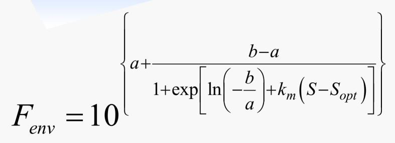
S = degree of saturation S = saturation at OMC  $k_m =$  regression coefficient a,b = constants (function of soil type)
