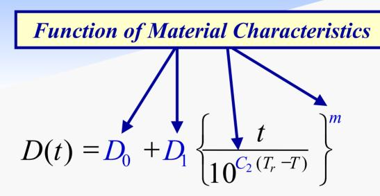
D(t) = Compliance t = time T = Temperature T<sub>r</sub> = Reference Temperature
