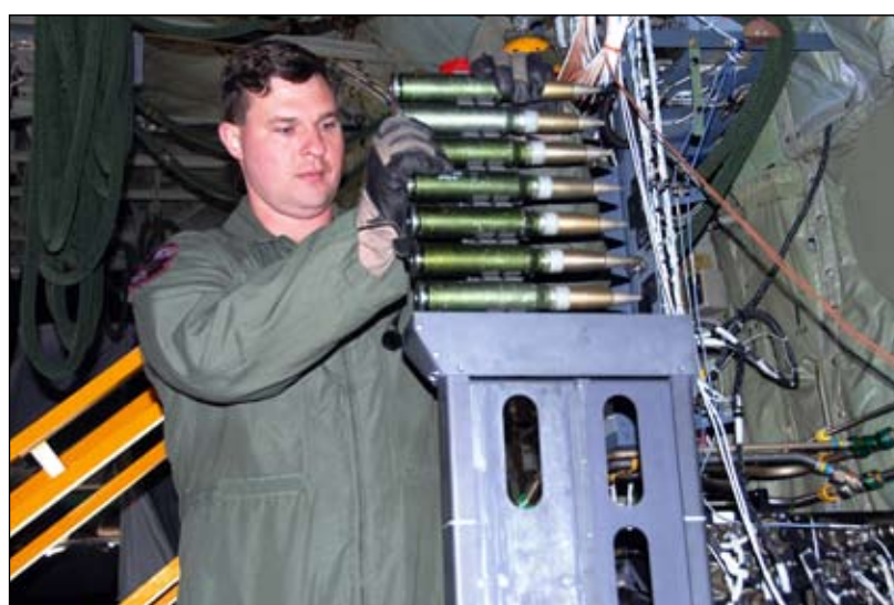
Tech. Sgt. Ben Filek practices loading a 30 mm Bushmaster cannon aboard an AC-130U Spooky gunship Jan. 26 at Hurlburt Field, Fla. The 30 mm gun will eventually replace both the 40 mm cannon and 25 mm gun on U-model gunships. Filek is an aerial gunner with the 19th Special Operations Squadron at Hurlburt Field.
