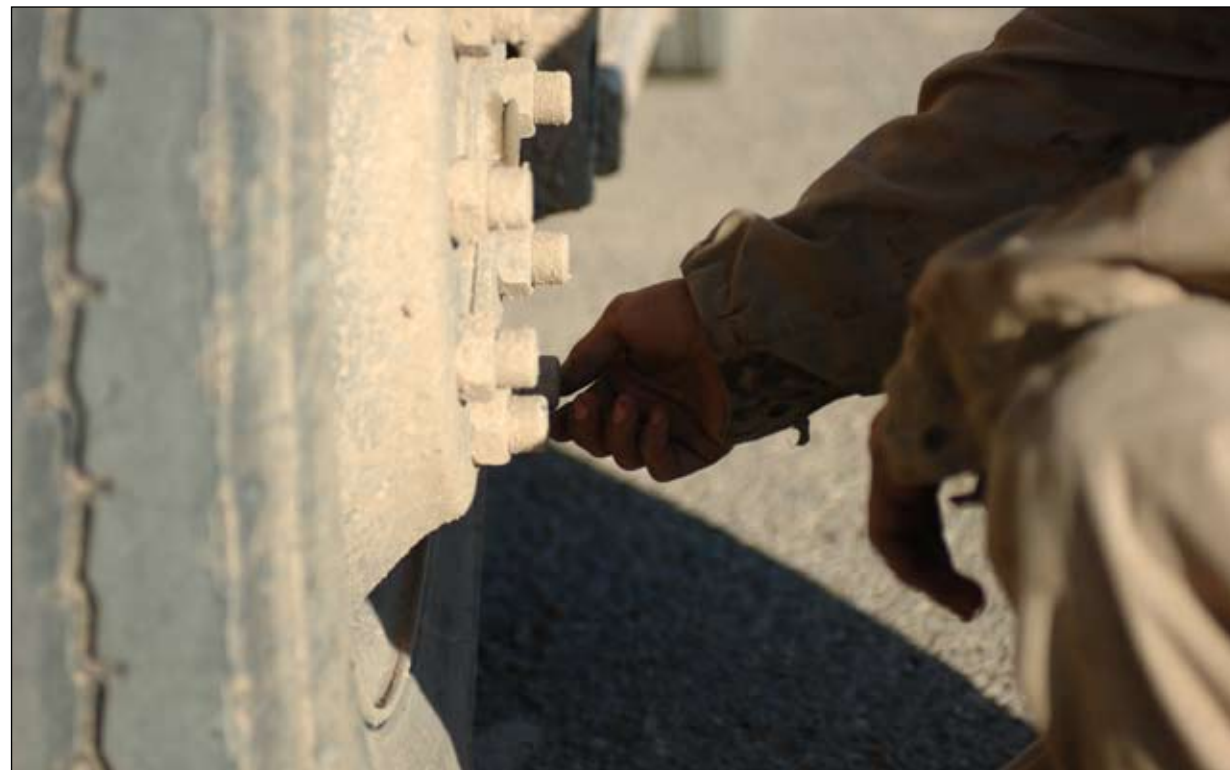
Spc. Michael Davis, a mechanic with 298th Trans. Co. checks the wheels on a M915 truck to ensure all the bolts are tight and the tires are properly inflated.
