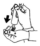
14. Push in bolt assembly to locked position.
