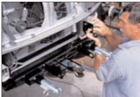
BASEPLATE INSTALLATION DOES NOT REQUIRE WELDING OR SPECIALIZED TOOLS. IF YOU HAVE ANY DOUBTS, HAVE A PROFESSIONAL DO IT.
