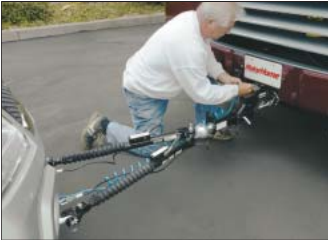
THE TOW BAR ATTACHES TO DINGHY QUICKLY AND EASILY WITH A PAIR OF HITCH PINS; TELESCOPING BARS FURTHER EASE THE HOOKUP.
