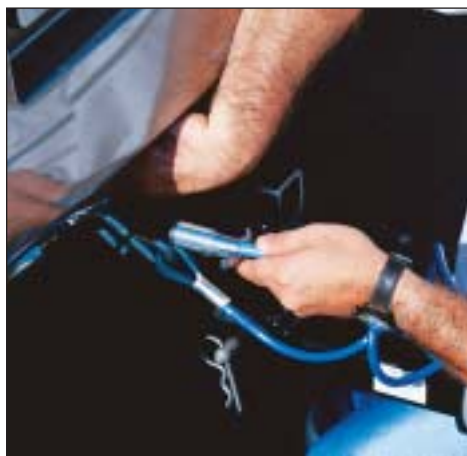
PLUG RECEPTACLES ADDED TO DINGHY AND MOTORHOME ALLOW EASY HOOKUP OF ELECTRICAL CONNECTOR FOR TAILLIGHTS, TURN SIGNALS AND SUPPLEMENTAL BRAKING SYSTEM.
