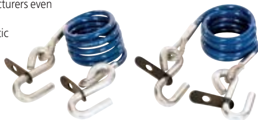
SAFETY CABLES ARE REQUIRED. INSTALLED, THEY MUST BE CROSSED TO CATCH THE TOW BAR IN CASE OF EMERGENCY.
