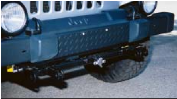
ONCE THE PROPER BASEPLATE IS INSTALLED, THIS CLEAN-LOOKING SETUP IS ALL THAT REMAINS WHEN THE TOWED VEHICLE ISN'T HOOKED UP; COOLING DOESN'T SUFFER.
