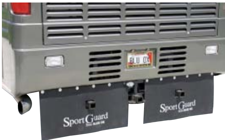
ADDING LARGE RUBBER FLAPS AT THE REAR OF A MOTORHOME WILL MINIMIZE TOWED-VEHICLE DAMAGE FROM DEBRIS, DIRT AND GRIME KICKED UP BY COACH TIRES.
