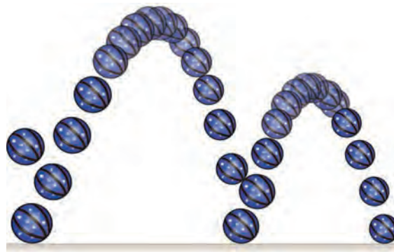
Fig 1.33: Each bounce of the ball is an inelastic collision.
