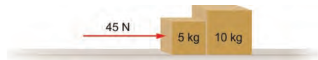
Fig 1.1: A 45 N force applied to a 5 kg block in contact with a 10 kg block
