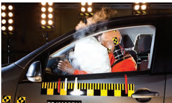
Fig 1.49: An airbag increases the time taken for the driver to come to rest during a collision
