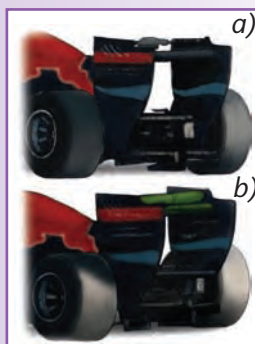
Fig 1.15: The drag reduction system on the rear wing is a) open and b) closed.
