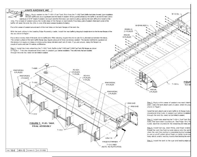
Above: An excerpt from an RV -10 plans page. Note the stepby-step construction sequences included on the same page as the drawings. Each part has a part number and is provided in the kit.
