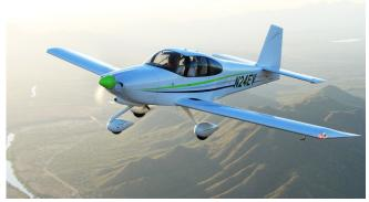
Occupant protection is an important concern. The composite cabin top provides roll-over protection. The cabin interior is designed around Oregon Aero seats and seat cushions, (provided in the kit) which provide the best available impact mitigation — and comfort. Like all other RVs, the RV-10 has impressively low stall and landing speeds. If necessary, it can be safely landed in very small spaces at speeds that give the occupants the best possible chance of escaping injury.
