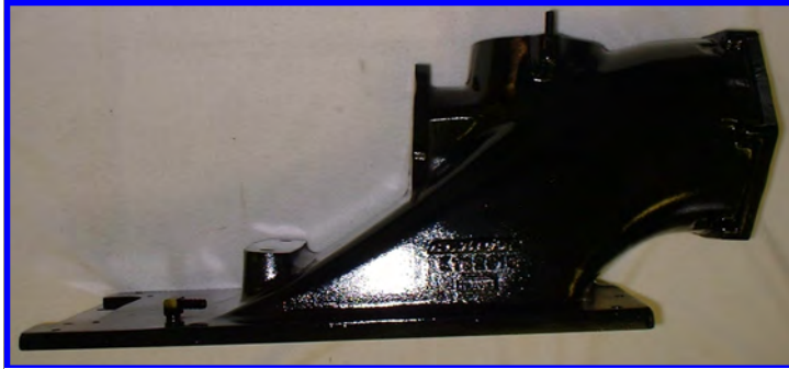
K702319 Main Intake Housing w/Wearing and Insulator Installed
