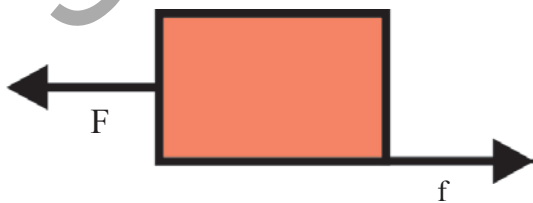
Fig-11: Horizontal forces on the brick
