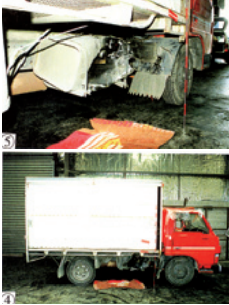
Results of a side underrun crash.
