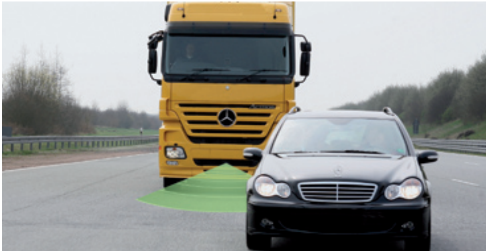
ACC sends out a beam that detects the speed and distance of the vehicle ahead.
