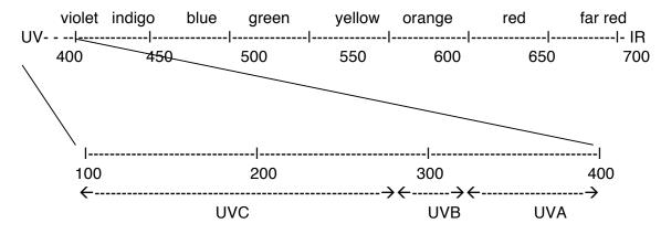
Light wavelengths between 100 and 400 nm are considered ultraviolet (UV). Wavelengths below 100 nm are extremely hazardous (i.e., ionizing radiations such as gamma rays and X-rays). Beyond 800 nm, the radiation is in the form of infrared (IR or heat rays), microwaves (10<sup>6</sup>-10<sup>9</sup> nm) and radio waves (10<sup>9</sup>-10<sup>12</sup> nm).
