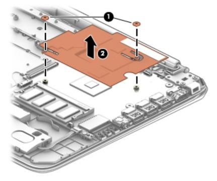
NOTE: The thermal material must be thoroughly cleaned from the surfaces of the heat sink and the system board each time the heat sink is removed. Thermal material is used on the processor (1) and the heat sink section (2) that services it.
