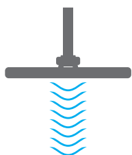
Front view of the Double-D strongest signal profile.
